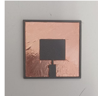
Figure 7: Example of one of the 3D printed patch antennas mould and cutting process.
