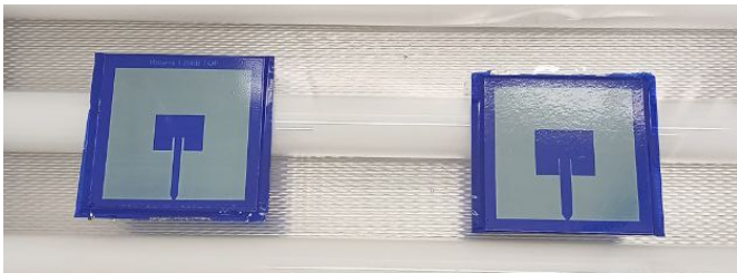
Figure 4: Two of the Rogers patch antennas after UV exposure.
