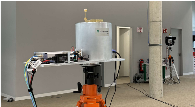
Figure 2: D-Band VUCA looking towards the TX.
