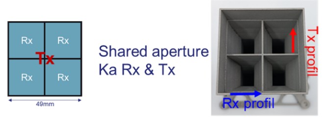
Figure 8: Concept of the shared-aperture radiating element with independent Rx and combined Tx paths.
