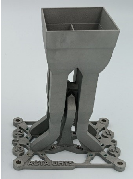
Figure 11: 3D-printed feed showcasing the Q-FPH design.
